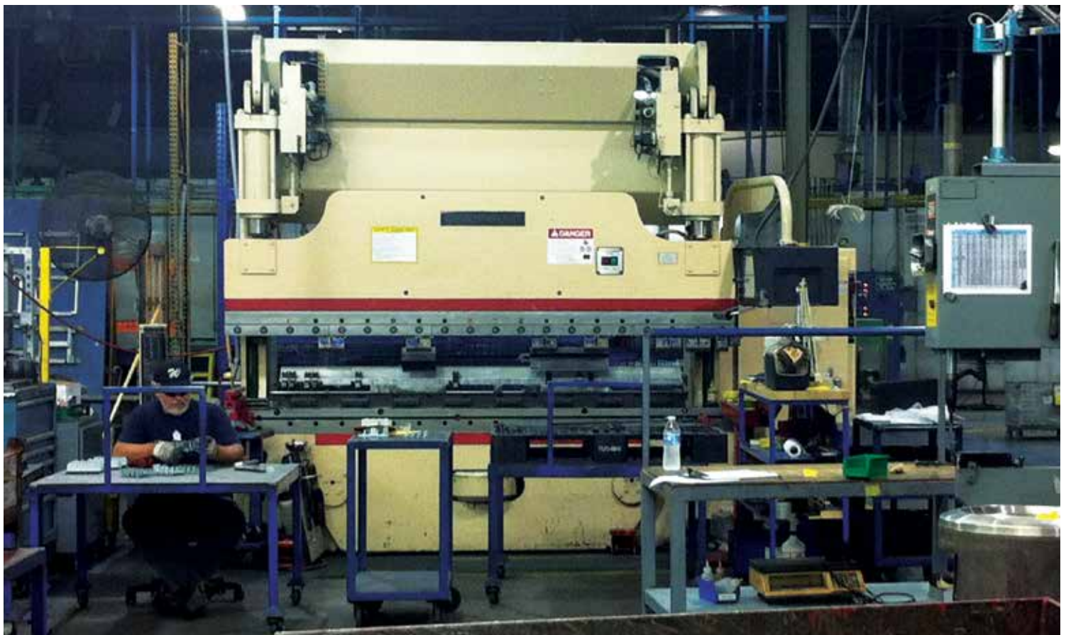
Technician Adjusting Parts for Metal Break Machine
